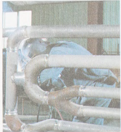
Finishing the fabrication of coil assemblies used in Canada's petrochemical industry. This operation combines machined sand-cast return bends with centrifugally cast tubing.
